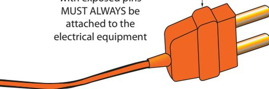
The half of the inline-connector that receives the pins from the other half MUST be attached to the part of the flexible cable connected to the plug
